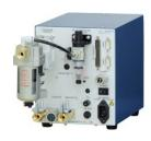
The leak tester's air-operated valves ensure reliable sealing and high flow rates. The basic circuit is the Intelligent 1 Pneumatic Circuit with excellent performance and reliability that checks valve operations and sensor sensitivity. The leak tester is also equipped with a function that prevents water, oil, and foreign matter adhering to the works from entering the measurement circuit.
